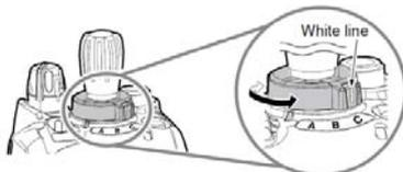
When the white line of the ABC switch is set to the position C, the pre-programmed function at position C will be activated.
